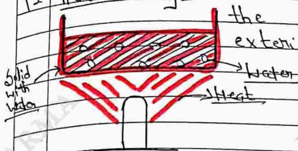
2. Mass transfer → It involves movement of the moisture to the surface of the solid and its subsequent evaporation from the surface.
