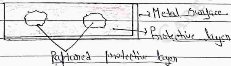
3) Structural Corrosion → In this type of corrosion, structural strength of metal get reduced due to corrosion.
